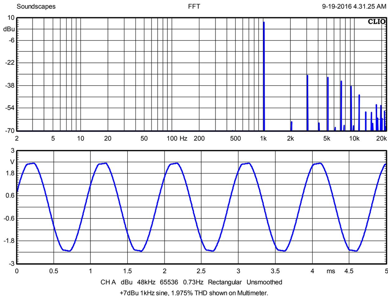
Fig 5: FFT of 1kHz sine at +7dBu drive level.
