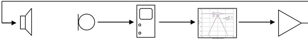
Fig 1: Loudspeaker (DUT), microphone, CLIO, digital processor and amplifier.
