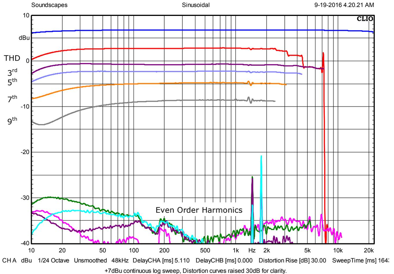
Fig 6: Sinusoidal module slow log sweep at +7dBu drive level with THD and harmonics raised 30dB for clarity.
